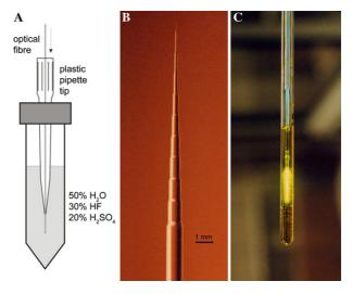
Fig. 2. (A) The production of the tapered fibre tip; (B) the resulting tip; and (C) an assembled NMR sample irradiated principally at 488 and 514 nm. The yellow colour is FMN fluorescence excited by the 488 nm laser line. The terminal diameter of the fibre cone is less than 50  $\mu$ m. In (C), the optical fibre appears much thicker than it actually is because of the lensing effect of the solution.
