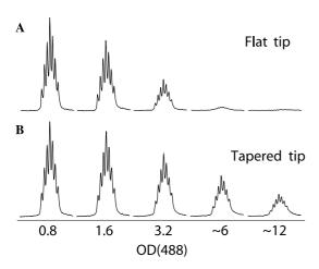
Fig. 5. <sup>19</sup>F photo-CIDNP signal amplitude as a function of photosensitizer concentration ([FMN] = 0.2–3.2 mM) for (A) illumination from above using the arrangement shown in Fig. 1D and (B) for a tapered fibre (Fig. 1F).
