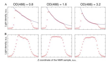
Fig. 4. The light intensity profiles along the z-axis of the sample measured using  $^{19}$ F photo-CIDNP of 4-fluorophenol ([FMN] = 0.2, 0.4, and 0.8 mM) for (A) illumination from above using the arrangement shown in Fig. 1D and (B) for a tapered fibre (Fig. 1F).
