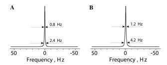
Fig. 6.  $^{1}$ H NMR lineshapes of the residual HDO signal in a sample of  $D_{2}O$ , (A) without and (B) with the fibre present inside the NMR tube. The field was reshimmed after the insertion of the fibre.
