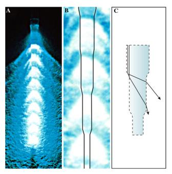
Fig. 3. (A) Emission of argon laser light from the tapered fibre tip placed on a white surface. (B) The central part of (A) magnified with the fibre outlined for clarity. (C) Likely paths of light rays in the fibre cone
